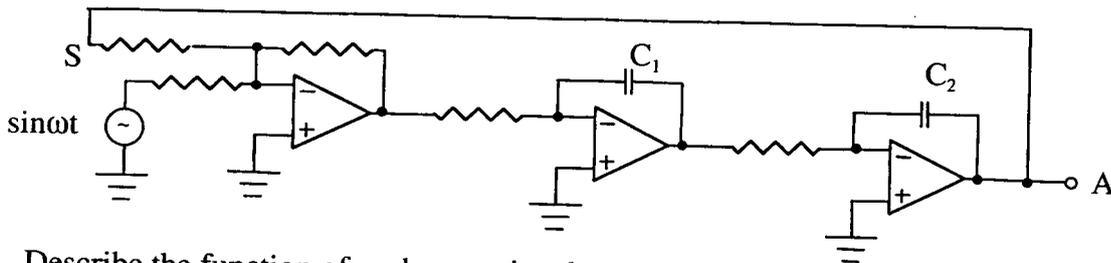
Describe the function of each operational amplifier section of the complete circuit and give their operational equations.
