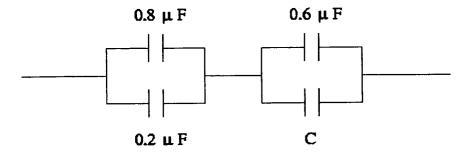
(c) Consider the system of two capacitors shown in the picture. Determine the magnitude of the voltage across each capacitor.
